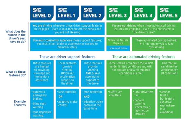
Fig 2.4 The SAE's 6 Levels of Autonomy
