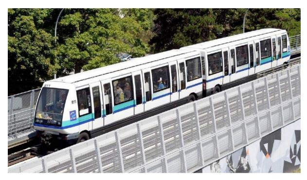
Fig 2.7 The Driverless, Rubber-Tyred, Rennes Metro
