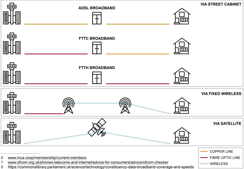
'Decent' broadband is delivered using a technology called **ADSL via copper cables** used by the telephone network. The majority of copper infrastructure across the UK is owned by Openreach with a small enclave around the Hull City Region owned by K-Com.
