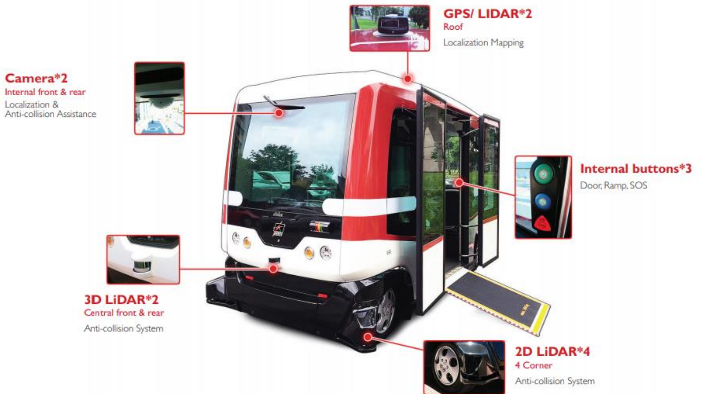
EasyMile EZ10 Detection and Navigation Technology [13]
