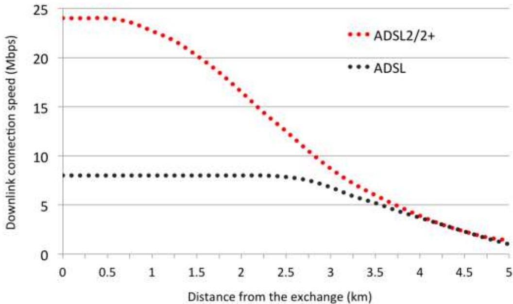
**Figure 2:** Relationship between estimated download speeds for ADSL and ADSL2 and the distance from the exchange [Source: Increase Broadband Speed]
