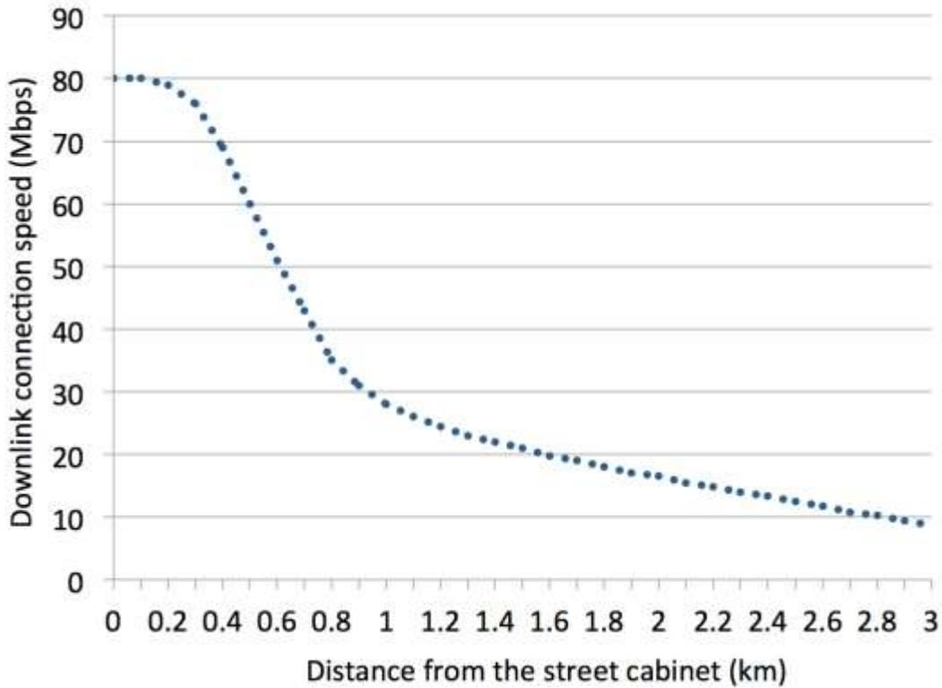
**Figure:** Relationship between download speed and distance from the fibre cabinet [Source: Increase Broadband Speed]
