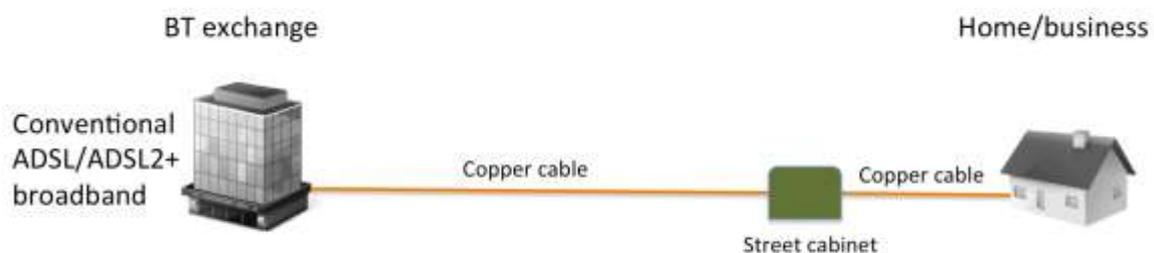
**Figure:** ADSL broadband is carried over copper cables between a BT exchange and premises
