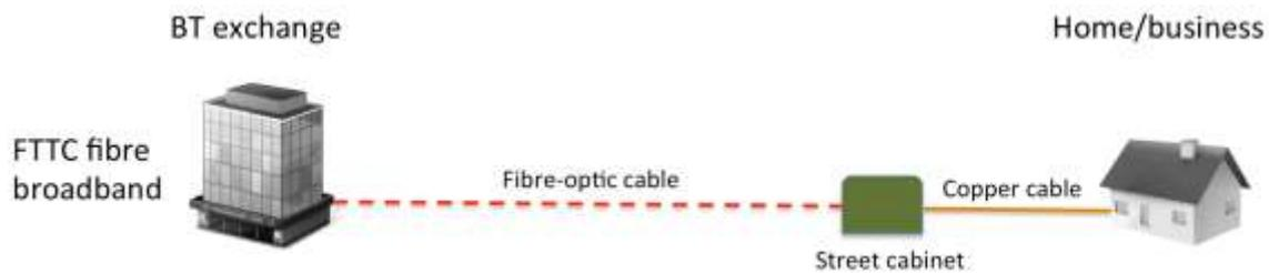
**Figure:** With fibre broadband, the distance that broadband signals have to travel over copper cables is substantially reduced compared with basic broadband
